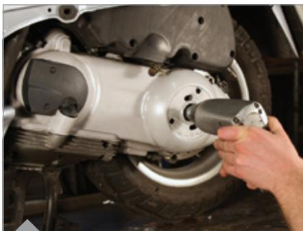
Remove the nut of the variator case with a 19mm socket or impact wrench.
