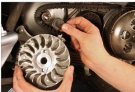
Don't forget the spacer that restricts the motor and is located between the variomatic and the ventilator disc.
