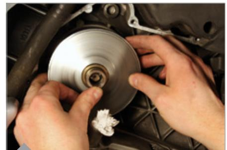
...and pull the variomatic carefully off the end – its off! During reassembly please make sure the variomatic is carefully pushed back into place to prevent any damage.
