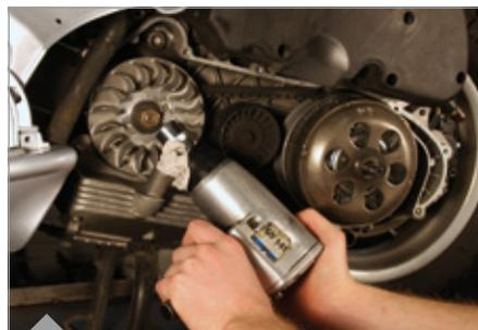
Now the nut holding the variomatic can also be removed with a 19mm impact wrench. In case you do not have an impact wrench, we recommend the use of a variomatic holding tool and a socket wrench.
