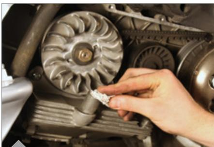
To avoid contamination of the motor's oil we recommend you plug the hole with a clean rag.
