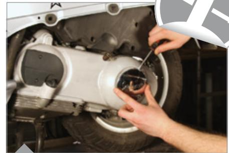
To remove the variomatic cover, the clutch nut trim must first be removed.
